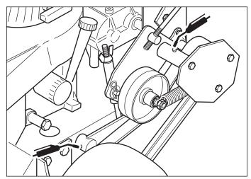
Figure 5. Brake Levers & Clutch Plate Pivots
